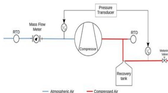
Figure 6 depicts a common compressor sensor configuration.
