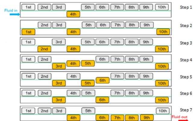
FIGURE 3: Schematic of a Mode 2 system with valve 4 and central piston 7.
