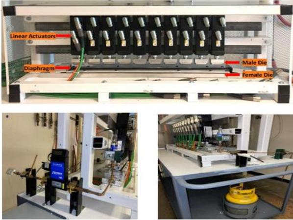
Figure 7: (a) Experimental prototype, (b) RTD, Mass-flow meter and Pressure transducer at inlet, (c) Pressure transducer, RTD and Recovery tank at outlet.
