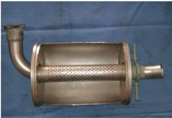
Fig 4: The resonator that was located on the back of the Tata Indica and was responsible for expelling the exhaust.
